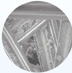
フィルター材 (Dillaとメルトブロン) Cross-section photo of Coarse Denir MARIX and MB nonwoven layered product (as reinforcement for filter)
